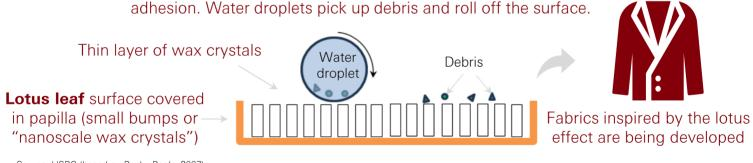
The **lotus effect**: a thin layer of wax crystals prevents water
